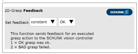
Depending on the quality of the grasping action performed, select "OK" or "Poor" as feedback. The return value can also be written via a register.
