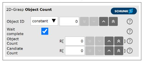
• Write the variable for the object class ID using the ID of the target object or select "0" for all objects.
